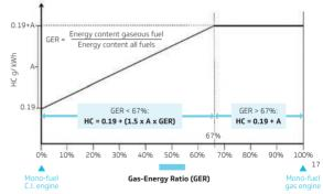
For sub-categories with a combined HC and NOx limit, the combined limit value for HC and NOx shall be reduced by 0.19 g/kWh and apply for NOx only.
