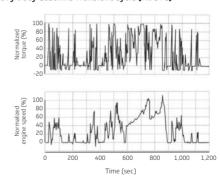
Test cycle comprised of 4 phases representing different driving conditions.
